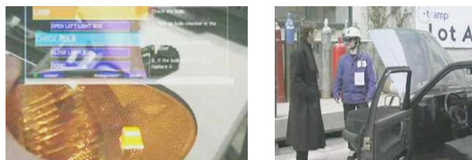
Figure 3: Augmented reality maintenance application. Left, mechanic's view through head-mounted display, showing step-by-step instructions. Right, mechanic with mock-up wearable computer. (Images from the TRAMP project.)
