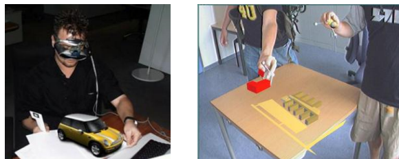
Figure 5: Left, automobile design: designer views model of vehicle through head-mounted display. Right, architectural design: virtual building is shown as it appears to an observer through a head-mounted display. (Images from the Fata Morgana [KDB + 02] and ARCHIE projects).
