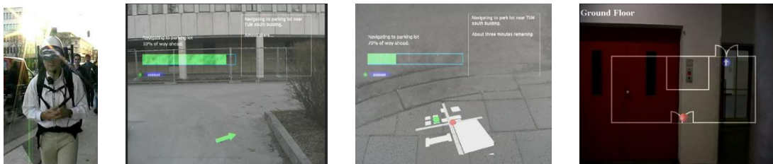
Figure 1: Mobile augmented reality: indoor and outdoor pedestrian navigation. Left, “wearable” prototype system; center, outdoor view through head-mounted display when user is looking straight and when looking down; right, view during indoor navigation. (Images from the TRAMP and Pathfinder [BBK + 01] projects.)
