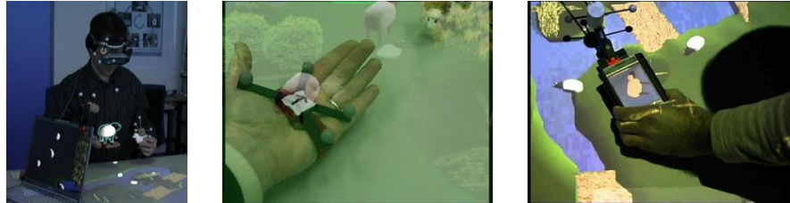
Figure 2: Augmented reality multi-player shepherding game. Left, virtual sheep floating on hand is shown on head-mounted display and laptop. Center, view through head-mounted display. Right, virtual sheep is scooped off projector table onto palmtop. (Images from the SHEEP [MSW + 03] project.)
